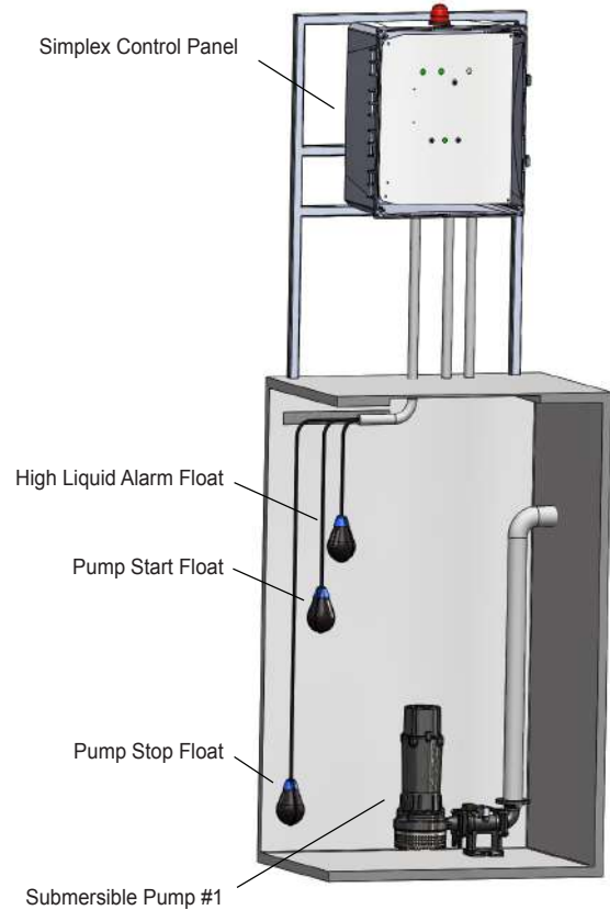
Typical Installation of Simplex Control Panel
