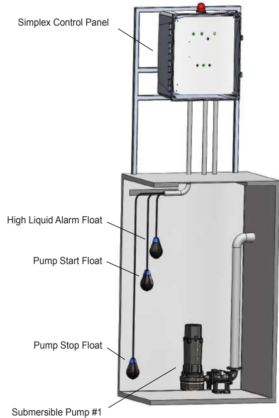
Typical Installation of Simplex Control Panel
